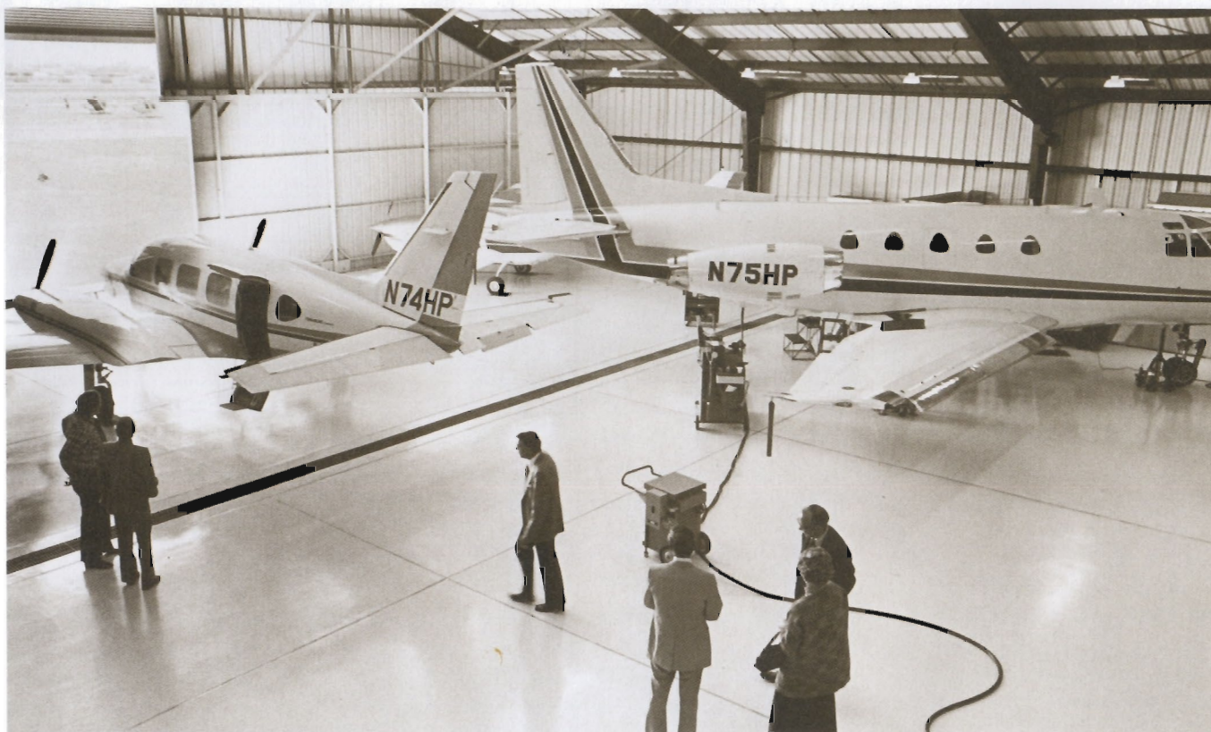
Visitors to the HP hangar, including the San Jose Airport Commissioners shown here on a recent tour, are generally amazed to see how clean everything is kept. The spotless floor even helped alert mechanics to a problem once, when spots from an oil leak appeared under the Navajo (left). On the right is one of HP's two Sabreliner jets.
